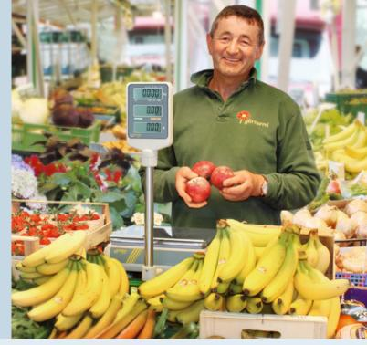
Price computing scales are used anywhere where the price of goods is calculated dependent on the weight of the goods. These scales must be  $\rightarrow$  verified in accordance with European Directive 2009/23/EEC. Usually, these scales are in verification class  $\boxed{\mathbf{M}}$   $\boxed{\mathbf{III}}$ .
